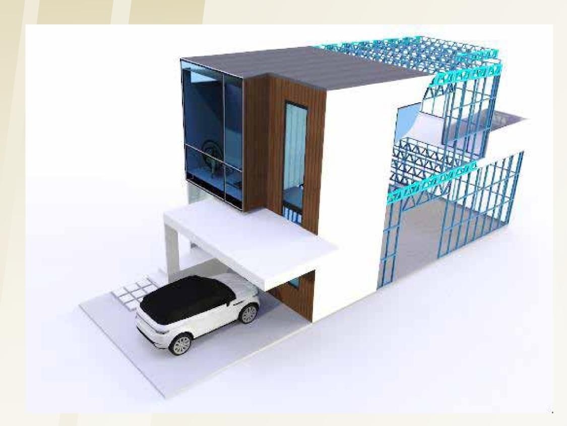
Dev<mark>elo</mark>ped the Lightrus Prefab System (based on proven Light Gauge Steel (LGS) technology)
